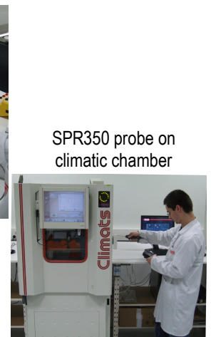
SPR350 probe on calibration oven
